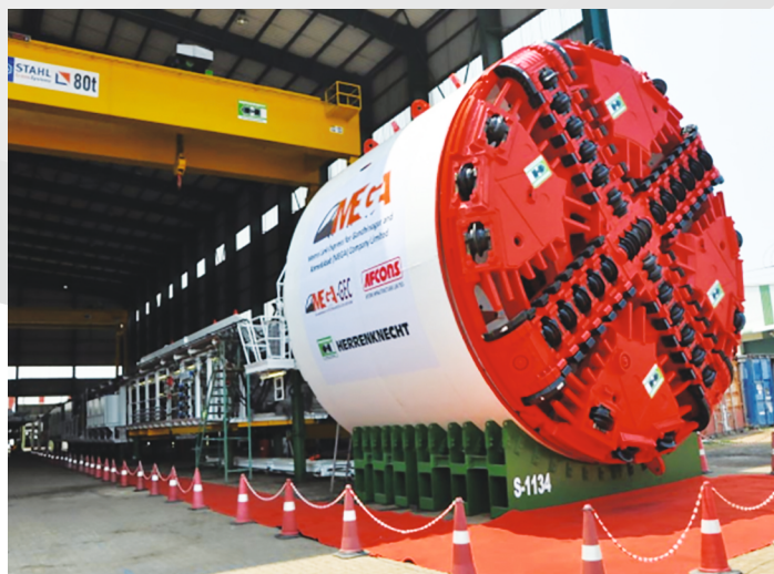
Fig. 1: Tunnel Boring Machine (TBM)
