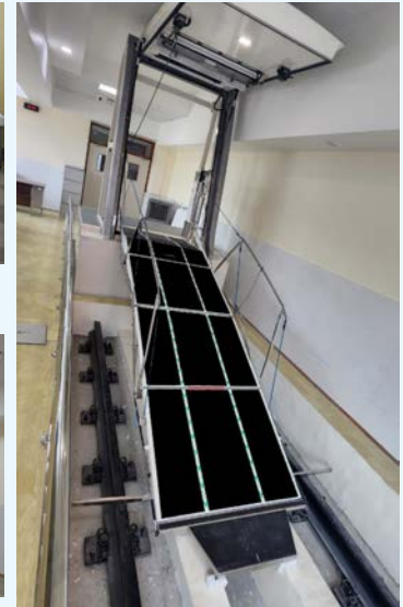
EMERGENCY DETRAINMENT DOOR
